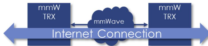
Figure 10: Internet connection using 60 GHz mmWave link.
