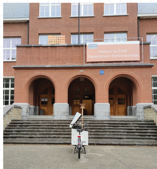
Picture 2: Rectangular array on the balcony of KU Leuven, with the bike-mounted mobile station in front
